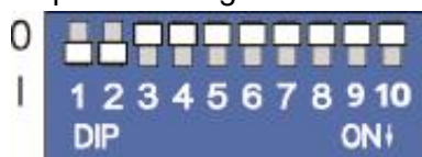
Figure 4: DIP switches (factory settings)
