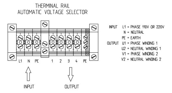
The shore earth <u>must</u> be connected with the gray input terminal marked PE. This wire may not be connected with the cabinet or any other therminal.
