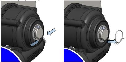
· Remove the key from shaft, the spring clip can be used to assist.
