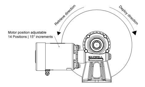
To ensure gearbox durability, position motor so that the input gear is at least partially covered with oil. Note: The diagram below has the drum winch mounted to the deck horizontally, if the drum winch is mounted to the vertical bulkhead the acceptable motor positions change accordingly.
