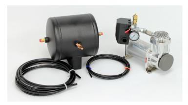
**Technical Details** Voltage: 12 V.D.C. (P449-17) Voltage: 24 V.D.C. (P449-34) Max Current: 21A @12 Volts, 12 A @ 24 Volts FAD @ 7 bar: ..85 CFM, 24 l/min Max Pressure: 150 p.s.i., 10.31 bar Weight: 14 lbs., 6.4 kg, Compressor and Tank Noise Level: 69 dB(A)@ 1 meter Thermal Protection: Yes Duty Cycle: 33% Vibration Isolated: Yes Wire Size: 12 AWG min.
